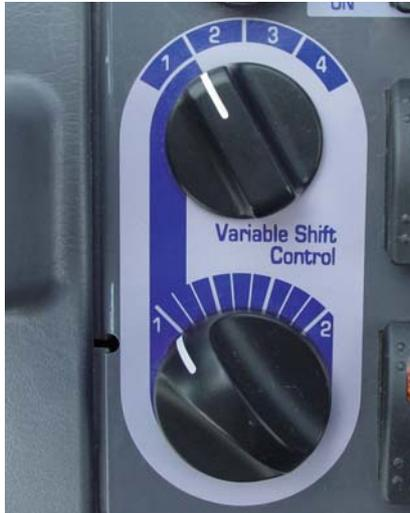
The variable shift switch allows the operator to adjust his machine speed in confined v-loading applications. When in 1, the operator can adjust his travel speed using the variable shift switch to match his machine speed and hydraulics to the distance he must travel.
