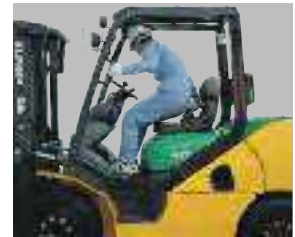
When the operator leaves the seat, OPS is activated
