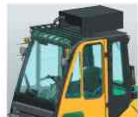
Steel cabin with cooler
